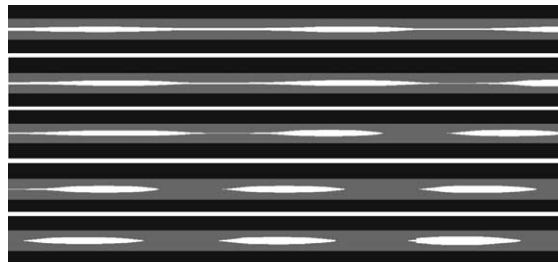
Fig. 9. Time sequence of the shape of an excited liquid jet and the emerging droplets for a situation where the jet decay occurs inside the capillary attached to the focusing zone.
