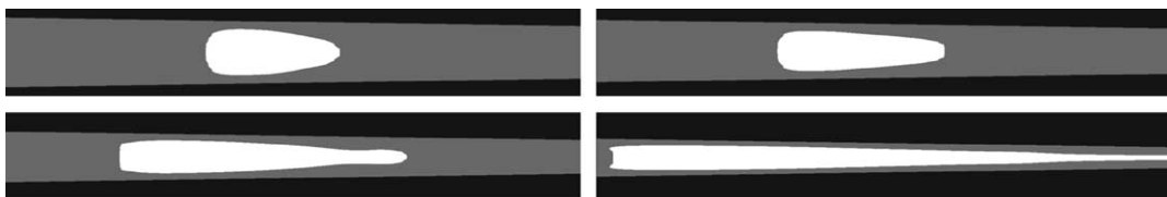
Fig. 10. Time sequence of a droplet having been created close to the entrance of the focusing zone and being stretched by hydrodynamic shear forces while convecting downstream.
